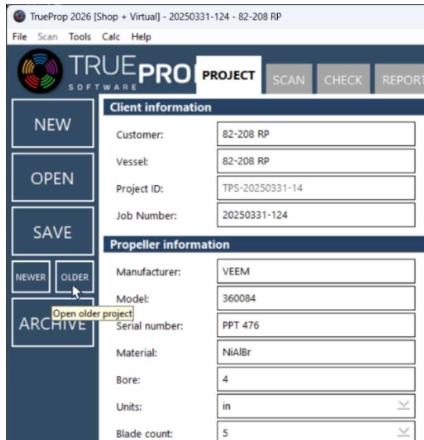
Figure 4: NEWER and OLDER project navigation lets shops move through active library projects faster, without returning to the full project list.
