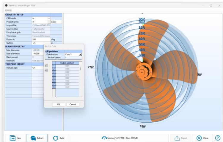
Figure 1: The Plugin automates geometric extraction from 3D scan models taken with any 3D scanner.
